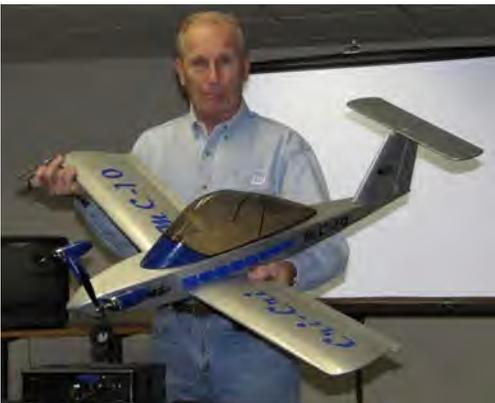
**Dean Copeland** displayed his recently built Chi Chi. Look closely and you will see two electric motors extending outward from the nose of the airplane. It is an ARF with a 46" wingspan that went together quickly. Chi Chi is French for Cricket. This model is a scale version of the real Chi Chi which a pilot fills up most of the area under the canopy in a crammed position. Dean's Chi Chi lacks being a true 1/4 scale model by 2" on the wingspan. Yes, the real McCoy is small.
