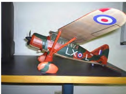
Master Builder **Jim Drickey** brought his Easy Built Model 1/12 scale Westland Lysander. This two-seat high-winged monoplane was famous for its nocturnal flights into occupied Europe, dropping supplies and agents behind enemy lines. Wingspan is 36 inches. It is an electric powered indoor flyer with GWS gear and a 4:1 brushed setup carrying an 800 mah lipo battery. This is an excellent example of Jim's building excellence. Phone [402-332-5955](tel:402-332-5955) to reach Jim.
